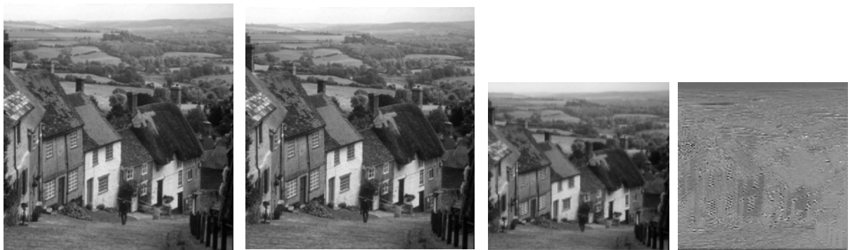
Original image Reconstructed image Approximation Details Fig. 13 The analysis and synthesis of Goldhill image using Daubechies-8 filter bank.
