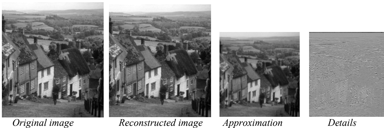
Fig. 9 The analysis and synthesis of Goldhill image using Daubechies-6 filter bank.
