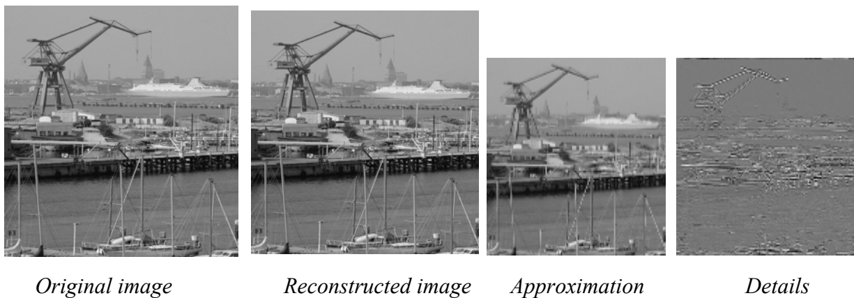
Fig. 10 The analysis and synthesis of Harbor image using Daubechies-6 filter bank.
