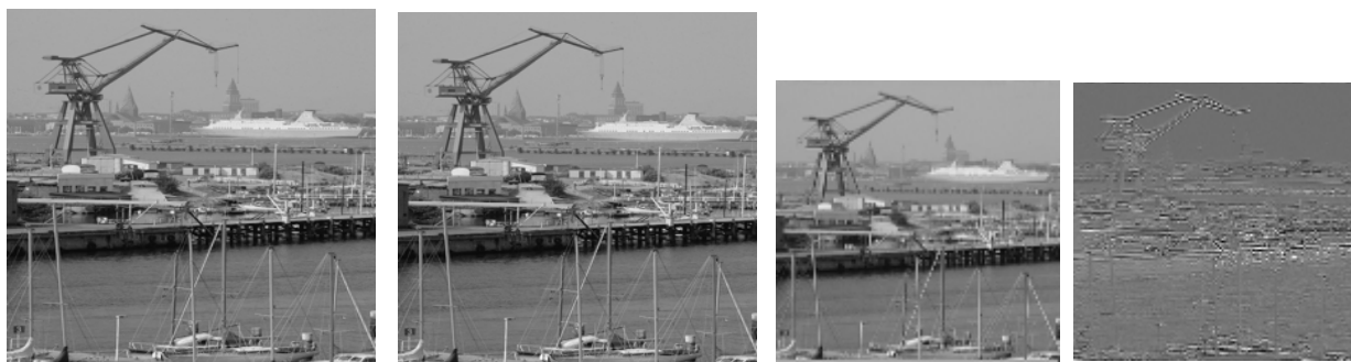
Original image Reconstructed image Approximation Details Fig. 14 The analysis and synthesis of Harbor image using Daubechies-8 filter bank.
