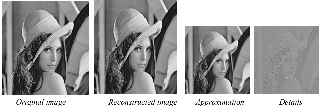
Fig. 8 The analysis and synthesis of Lena image using Daubechies-6 filter bank.
