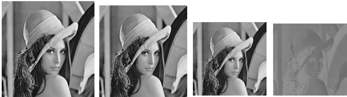
Original image Reconstructed image Approximation Details Fig. 12 The analysis and synthesis of Lena image using Daubechies-8 filter bank.
